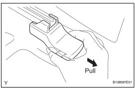
(d) After the 2 claws have been removed, carefully pull the front seat track cover rearward and remove the front seat track cover.
