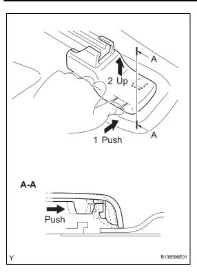
(c) Lift up on the area where the claw was removed. Then push in the direction of the claw on the opposite side to remove the outside claw.
